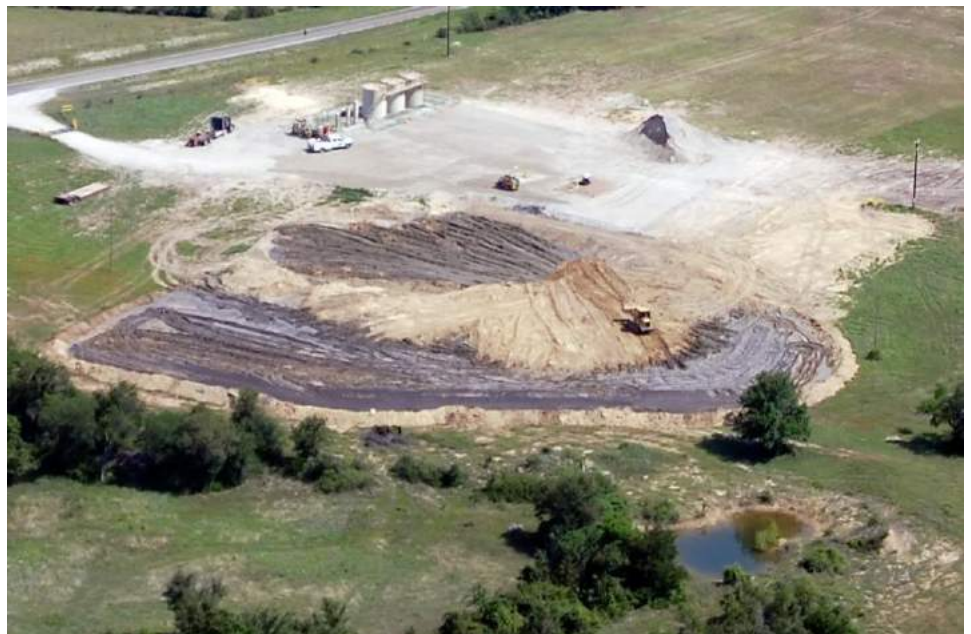
Fracking well site with condensate tanks, landfarming and adjacent wastewater pit. Wade County, Texas. Photo: Bluedaze.
