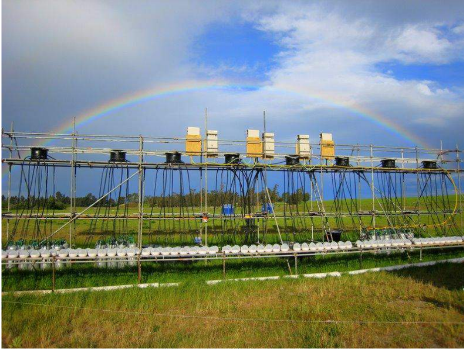
An experiment under the rainbow – The Kauru stream channel experiment. A complex set-up comprising 128 circular stream channels, 8 water temperatures, 2 nutrient levels and 2 deposited fine sediment levels. Photo: Jeremy 'Jay' Piggott.
