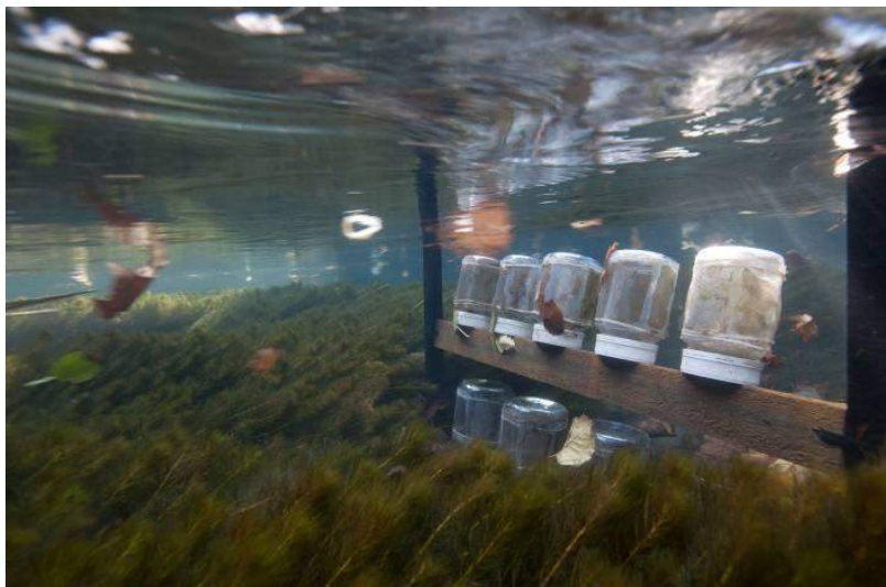
Bioassay cages at the upstream control site in the Avon River. Photo Shelley McMurtrie
