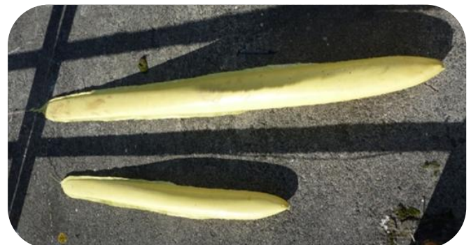
Urethane rubber model eels used in the spillway trial. Small eel dimensions: 1 m long, maximum diameter 100 mm, weight approximately 4.5 kg.
