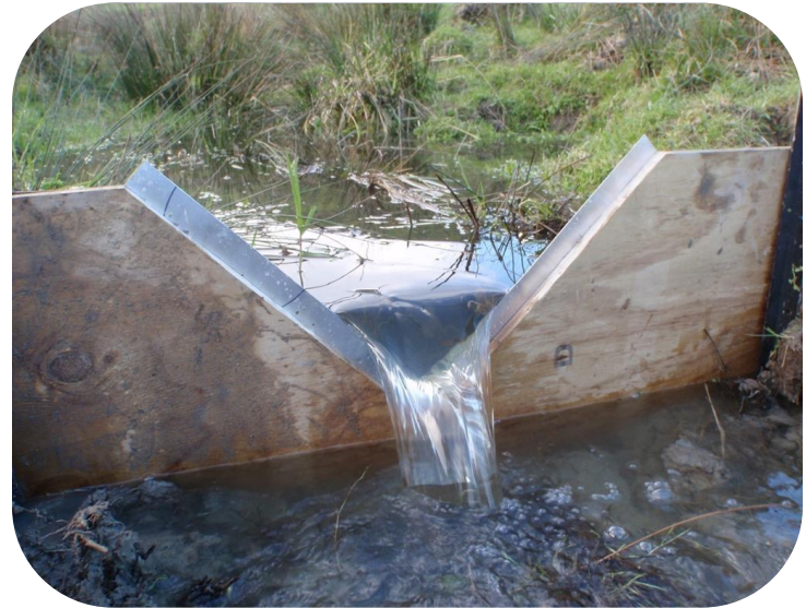
Small stream gauging using a portable V-notch weir as part of the Te Māhia Beach Wastewater Scheme baseline water quality and aquatic ecology survey. Photo: Olivier Ausseil.
