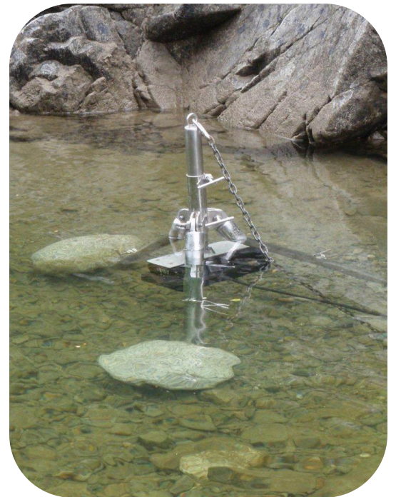
The DIDSON set up in the Mokihinui to monitor eel migration during flooding. Photo: A. Quarterman
