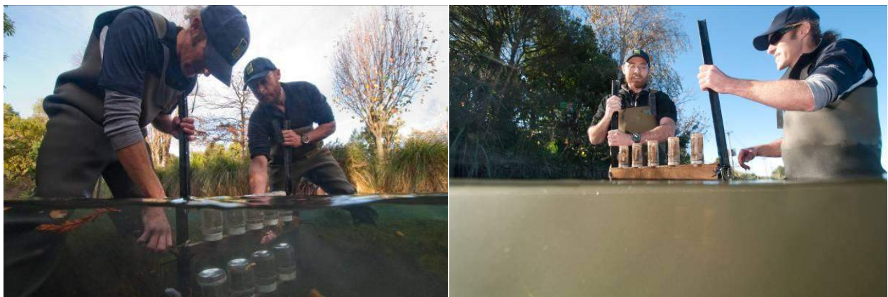
Removing invertebrate bioassay cages in the Avon River upstream (left) and downstream (right) of sewage inputs. Photos: Shelley McMurtrie
