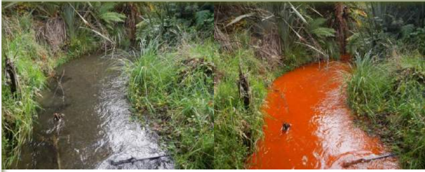
“Colour-in our rivers”: Rhodamine release in 22 Waikato’s streams to assess differences in DO between fenced and unfenced stream reaches as part of the MBIE (formerly MSI) Aquatic Rehabilitation Project. Photo: Kati Doehring
