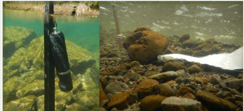
An optical sensor measuring dissolved oxygen to determine rates of stream metabolism (left) and a cotton strip deployed on the stream bed to determine cellulose decomposition potential in streams (right). Photo: Annika Wagenhoff
