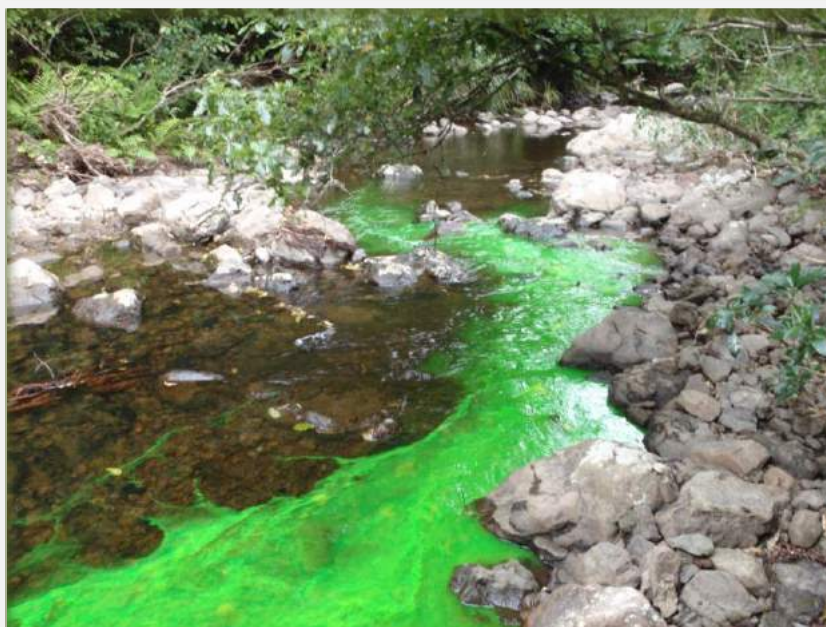
Dye (fluorescein) testing: an easy way to check travel times and lateral mixing. Turitea Stream, downstream of the point of backwash water discharge from Palmerston North's potable water treatment plant. Photo: Olivier Ausseil.
