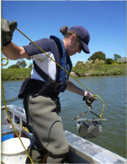
Top: Alex James, Amber Sinton and Shelley McMurtrie measuring a large anaesthetised longfin eel caught in the Avon River. Photo: EOS Ecology/Bronwyn Gay. Bottom: Nick Hempston collecting a ponar grab sample in the lower Avon River. Photo: EOS Ecology.
