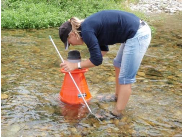
Kati Doehring using the periphyton viewer (one of the five sediment protocol methods) to assess fine particle sedimentation. Photo: Joanne Clapcott
