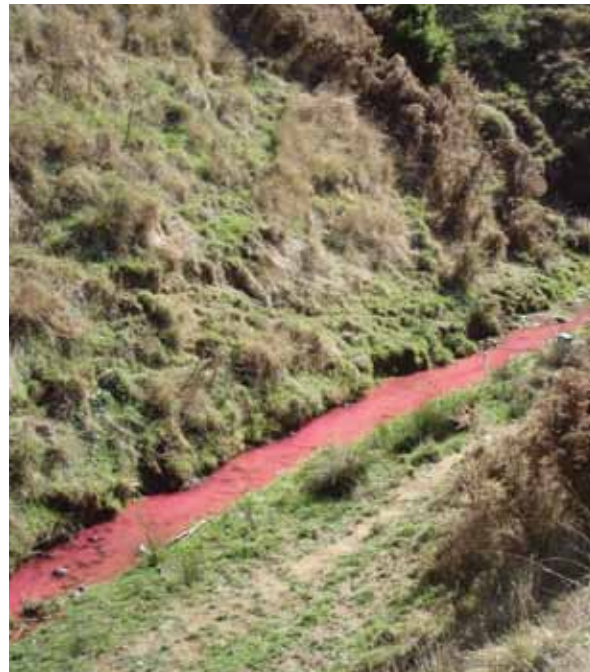
Dye addition experiment to determine retention time with, and without wood at the lower Keripaka Stream site.
