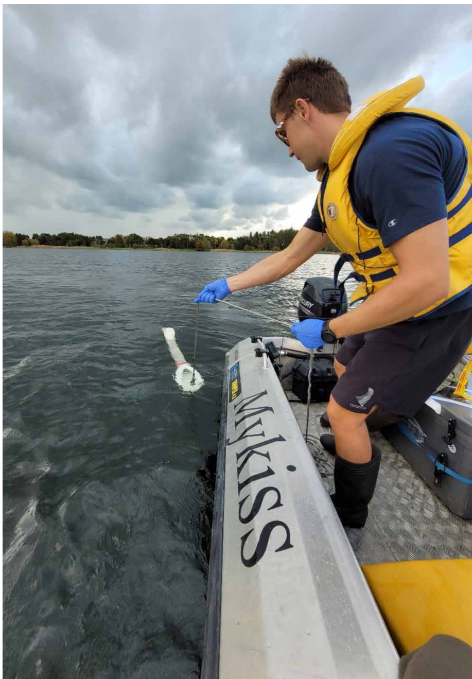
Photo: University of Waikato MSc student Ashton Reiser using a Cruising Speed Net sampler on loan from Xavier Pochon (Cawthron Institute) to collect eDNA samples from Lake Puketirini. Photo credit: Kerry Bodmin (DOC)
